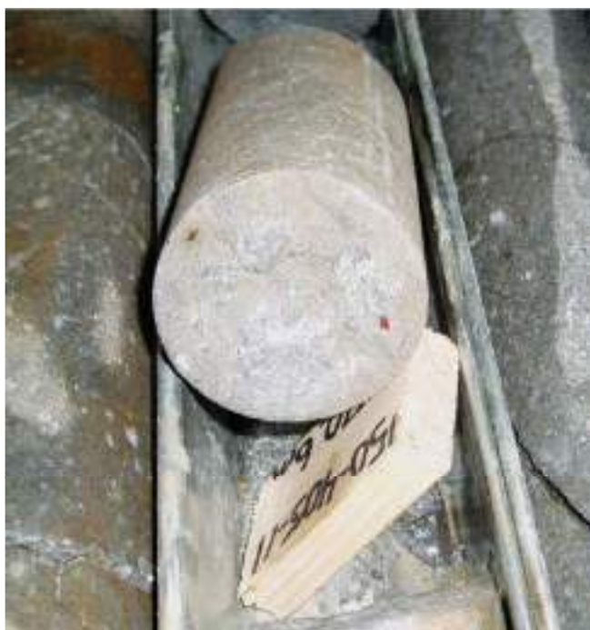
FIG 6 - Example of a very discrete orientation mark near the edge of the core. This mark was allegedly made by a spear but is more likely to have been fabricated.
