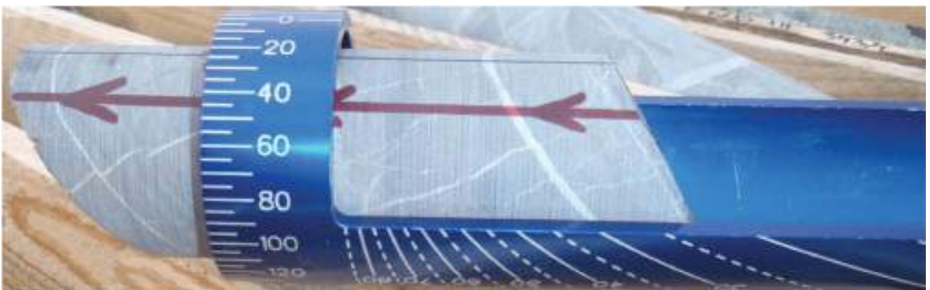
FIG 17 - Oriented core inside a Kenometer™. This device allows for easy measurement of alpha and beta angles.
