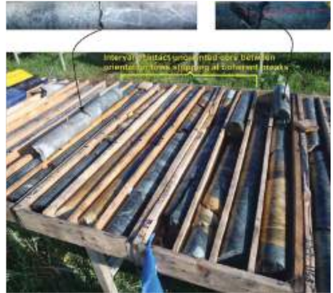
FIG 14 - Example of high-confidence orientation lines terminating at core breaks that could be confidently reassembled. The breaks are shown in the oriented core with the orientation lines at the top of the figure. Terminating the lines has meant that a large interval of coherent core has not been oriented. In this case, the lack of orientation line was a concern because the unmarked interval contained a number of important structures needing to be measured.
