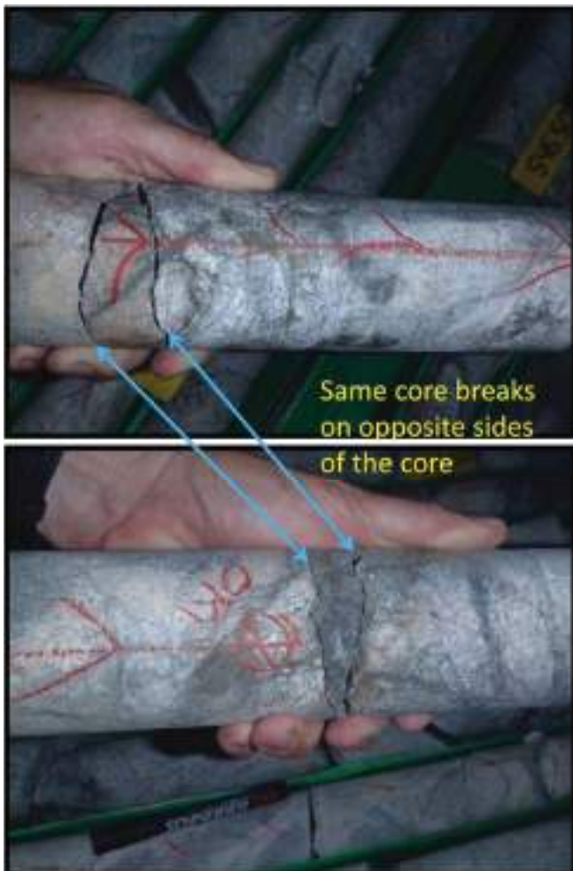
FIG 13 - An example of a dislocated orientation line that is hard to explain. Either the core had not been diligently reassembled, or the orientation line had been drawn from two different directions and did not match. In both cases the orientation lines are of no confidence.
