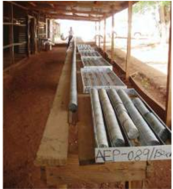
FIG 8 - Core laid out in a piece of angle iron to the left of the trays from which it was taken. The oriented marks are then lined up and the edge of the angle iron used as a guide to draw the orientation line.
