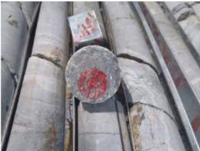
FIG 4 - The poorly designed spear in Figure 2F has produced the mark shown here. The orientation mark was originally a yellow spot but the mark has been overwritten by drillers trying to be helpful through painting around the mark. Both the state of the spear and the mark should have been identified by the geologist in charge and rectified.
