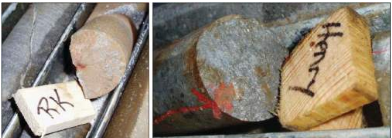
FIG 5 - Examples of driller identification on core blocks at the break where the orientation was taken. RK has produced an unusable mark whereas Henry has produced a good mark.
