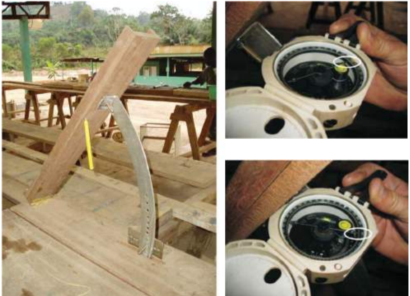
FIG 16 - Examples of problems arising from a core frame that contains magnetic material (left). The yellow item is a pen magnet. The upper-right photo shows the compass several centimetres away from the core frame, whereas the lower one shows the compass resting against the core frame. The two photos show that the needle orientation in the compass can be out by as much as 30°, depending on proximity to the core frame.
