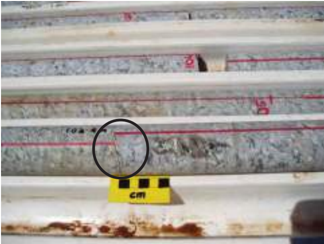
FIG 7 - The core either side of the angled break (circled) fits together tightly.
