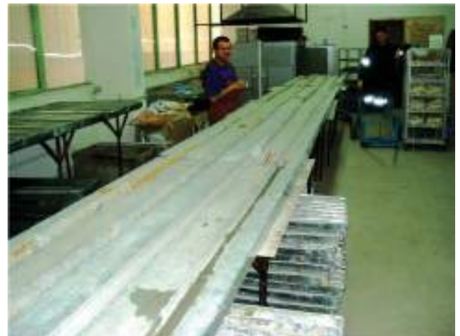
FIG 9 - Core laid out on a sheet of iron with angular corrugations. The orientation marks are aligned on the top side of the core (still bottom-of-hole but the core is rotated around). A piece of iron is then rubbed against the core and produces a non-temporary line on pieces of adjacent core. This line can then be checked against the marks for consistency and over-written in ink if the marks are of good quality.
