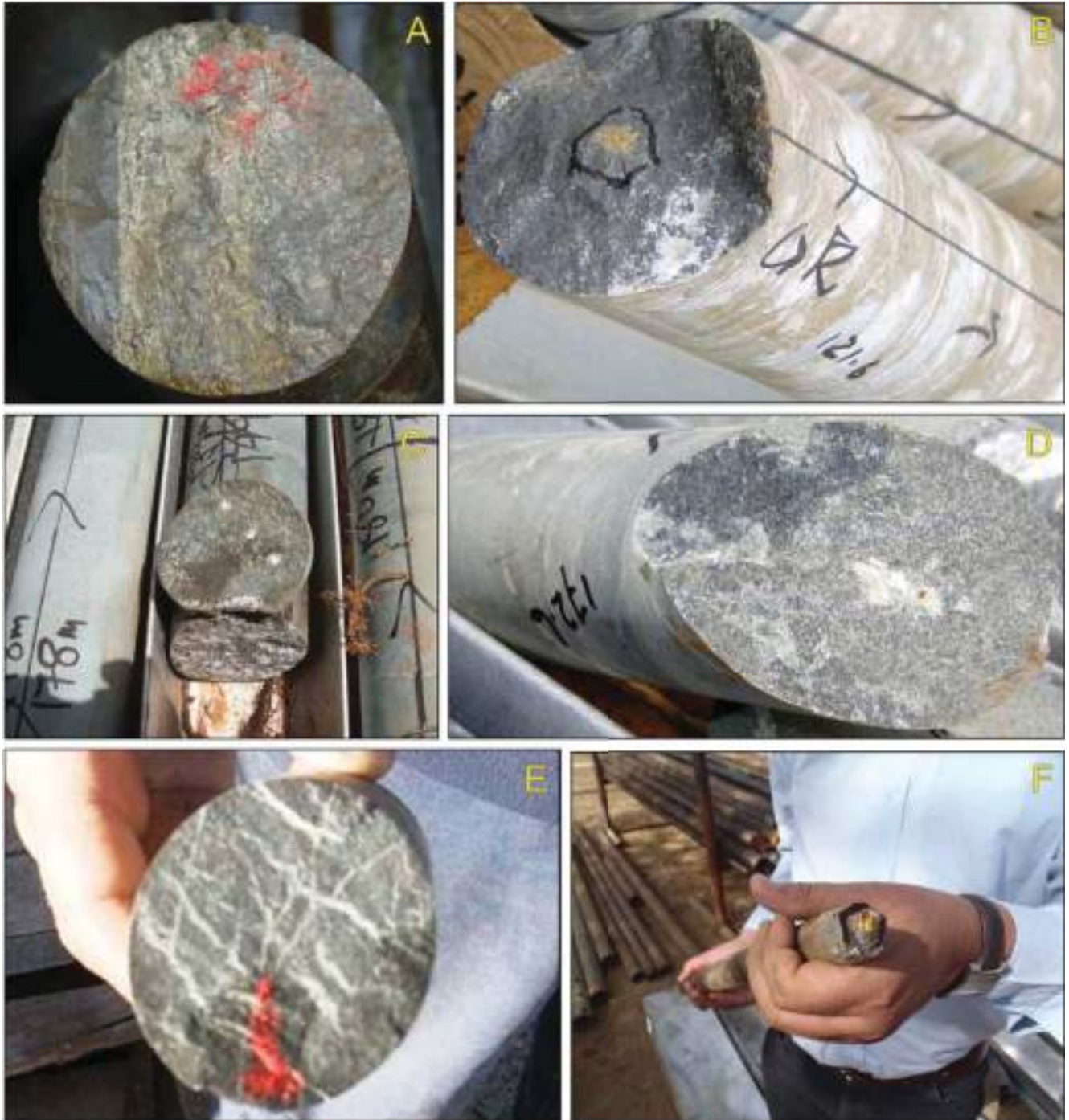
FIG 2 - (A) to (E) show various marks made using a downhole spear that has had either a hardened metal tip or a crayon tip. (A) Smeared crayon mark defining a poor quality orientation mark, which is too wide to confidently locate the bottom-of-core position. (B) Unusable mark produced by a metal-tipped spear in the centre of a core interval. (C) Several metal-tipped spear impact marks at various positions across a core break. The impact marks define a line and are a result of dropping the spear from too far up the hole. (D) Elongated metal-tipped spear impact mark defining an unusable orientation mark in the centre of the core break. (E) Smudged crayon impact mark. Although the inclination would be to use the point at which the mark intersects the edge of the core, this is not correct and the mark should be treated as unusable. (F) Example of a poorly designed spear comprising an impact tip of a blunt crayon loosely attached to the spear with gaffer tape.
