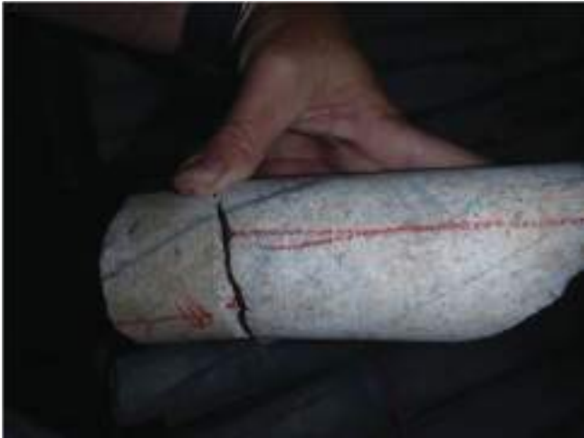
FIG 12 - Poor geological practice exemplified by misalignment of a core orientation line across a core break. Note that the core fits together well, and when it does the pyritic vein under the thumb is continuous.
