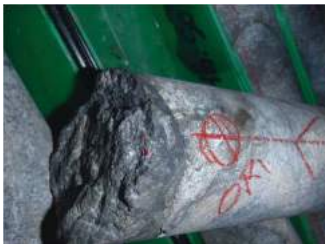
FIG 15 - 'Oriented' core showing a red downhole spear orientation mark on the core break. The core break represents the start of a new core run and progressively deeper portions of core are located in a direction away from the mark. Consequently, the orientation line on the outside of the core that points towards the orientation mark is incorrect because it indicates an uphole direction.
