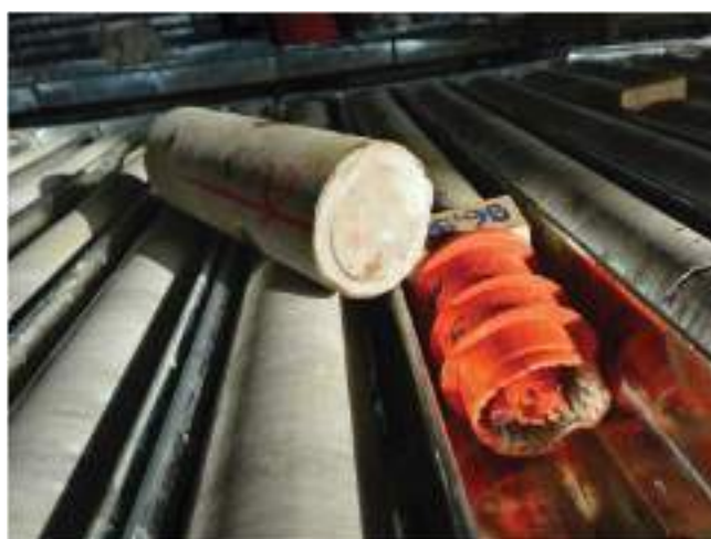
FIG 11 - Example of a portion of core showing evidence for core-spin. The spin marks were due to the rotation of core from the previously drilled interval. The piece of core in this figure represented the start of a new core run and did not undergo rotation.
