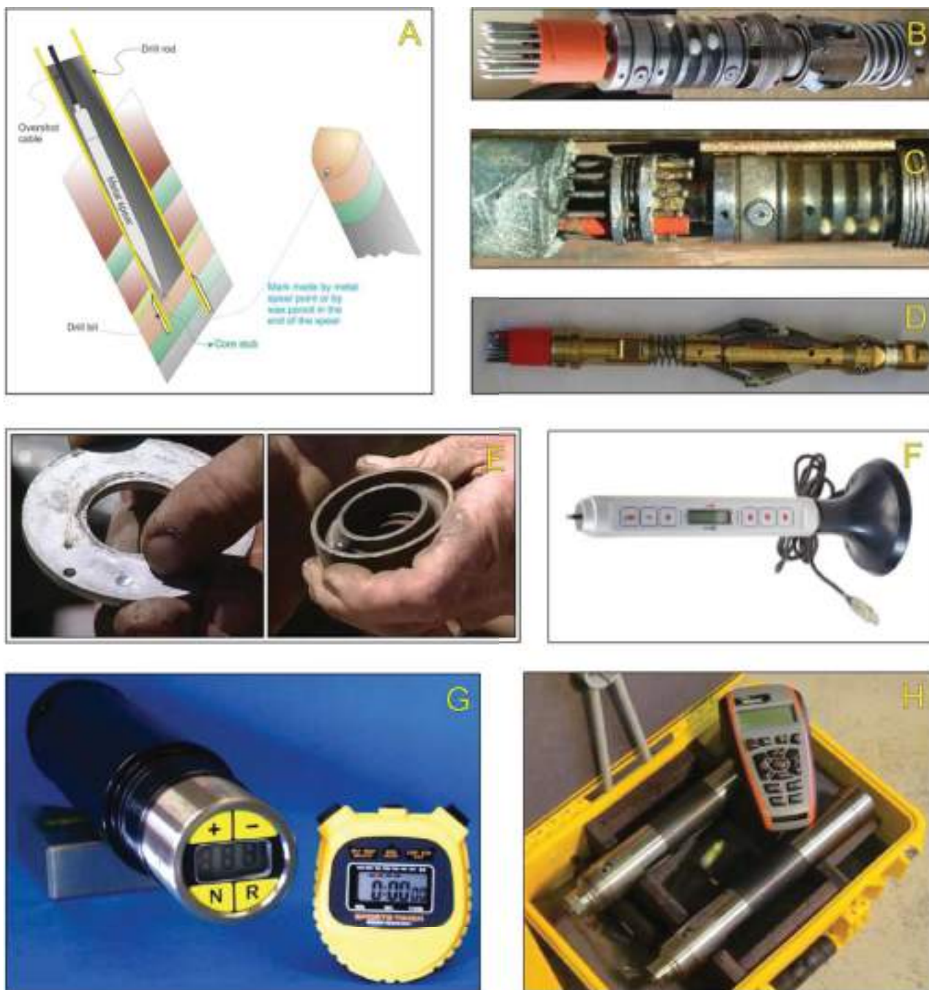
FIG 1 - Examples of various diamond core orienting tools. (A) The downhole spear. (B) The Ezy-Mark™ tool. The orange section has pins that conform to the shape of the core stub, as seen in (C) below. The orange section can be left in the core tray as a proxy for a core block, thereby preserving the orientation with the core. (C) Ezy-Mark™ tool with permanent pins and crayon. Note the three aligned balls on the right-hand side of the instrument. (D) The Verti-Ori™ tool. (E) Ballmark® soft metal washer (left) with reference mark (hole) and orientation indentation (near finger). The right-hand picture shows the ceramic ball in the track where it freely rotates until the orientation is made. (F) The Reflex™ tool. (G) The Ace™ tool (left) and stopwatch (right). (H) The ORIsht™ tool showing orientation instruments and handset.
