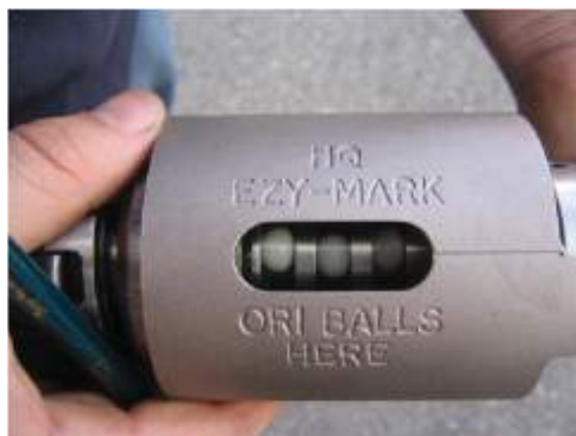
FIG 3 - Orientation shroud for the Ezy-Mark™ tool showing viewing window where a high-confidence orientation mark is indicated by the alignment of the three balls.
