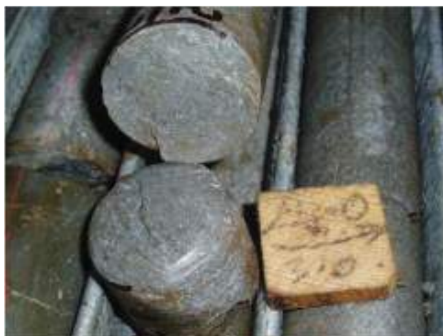
FIG 10 - Example of core spin that has induced circular marks on the core either side of the break.
